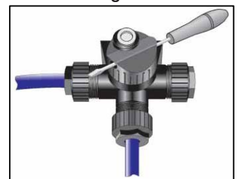
Figure 5: Always ensure that the connectors are firmly tightened. This shows a Siemens PROFIBUS PA connector being tightened using a screwdriver.
